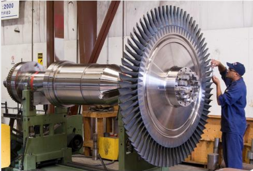
Example of a 45MW hot gas expander working at 760° C (source ELLIOTT company)
