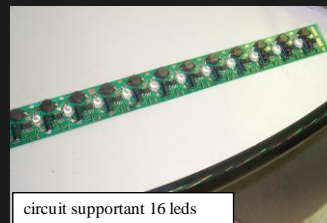
circuit supportant 16 leds
