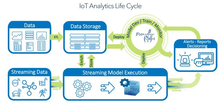
Figure 5: The IoT analytics life cycle - stream it, filter it, score it and store it.
