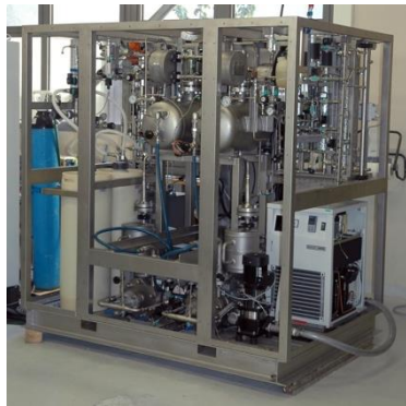
Electrolyser PEM 10 Nm 3 /h – 50 kW
