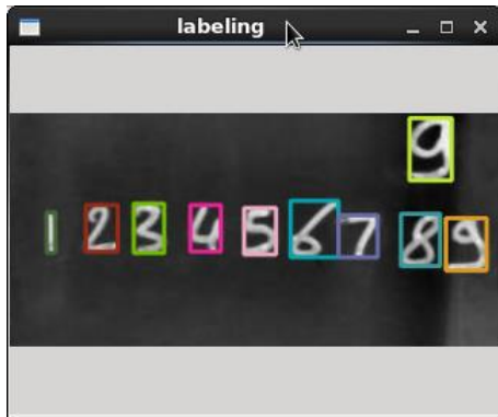
1) Plates extraction, perspective correction and segmentation
